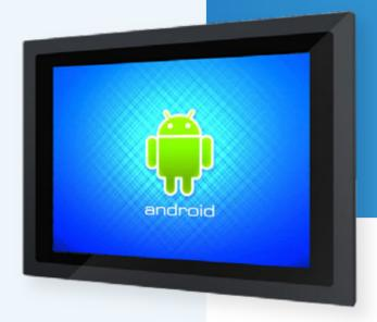
EPC-410 Android is a cost effective and compact Panel PC for any Industry 4.0, IoT, Automation and Digital Transformation application which requires Android platform with its Quad Core ARM Processor, rich I/O and robust aluminum die casting chassis.
