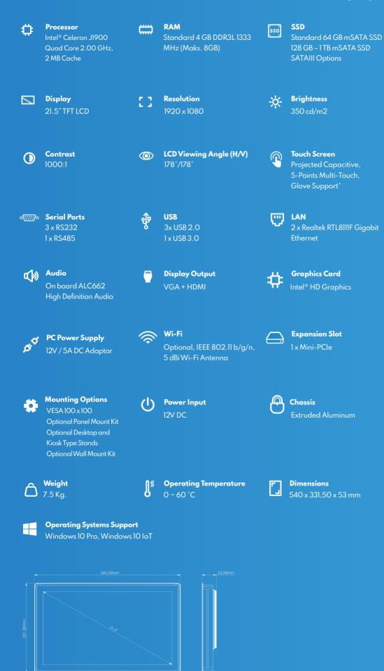
Technical specifications may be changed by Noya Dijital Dönüşüm Teknolojileri A.Ş at any time without prior notice or explanation to the us 'Touch Screen glove support is valid for Latex, PVC, Nitrile and PU gloves.
